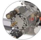
Main motor with leak-oil connection
